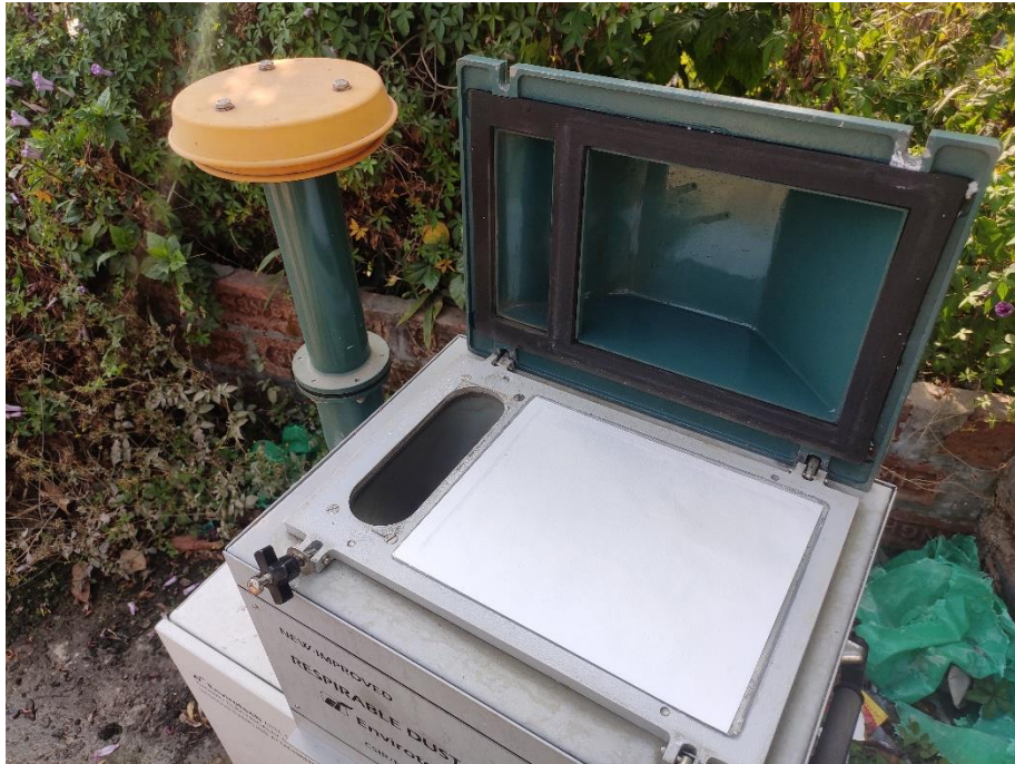
Plate 3 (a): Inner Section of the Respirable Dust Sampler with new filter paper before operation
