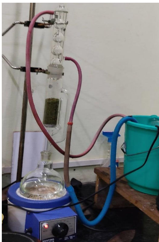
Figure 3: Extraction of plant specimen using Soxhlet apparatus for phytochemical analysis.
