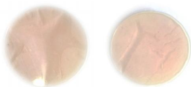
Figure 9: Change of yellow colour impregnated filter paper into reddish brown due to the production of HCN
