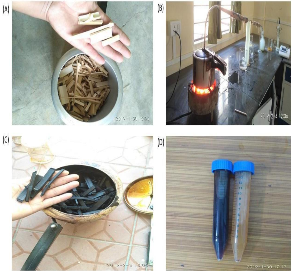
Photo plate 6: Extraction of pyrolyzed bamboo liquid (vinegar), (A) Pieces of bamboo culm, (B) Improved pyrolysis units, (C) Bamboo biochar after the pyrolysis and (D) Extracted vinegar
