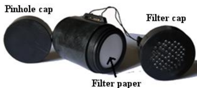
Figure 2.1 BARC type twin cup dosimeter.
