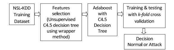
Figure 4.1: Block diagram of proposed hybrid network intrusion detection system.
