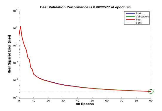
Figure 3.9: Performance of stage-2 classifier with 40 hidden layers at 90 epochs.
