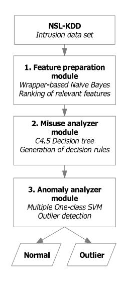
Figure 5.1: Proposed hybrid detection technique fusing misuse and anomaly technique.
