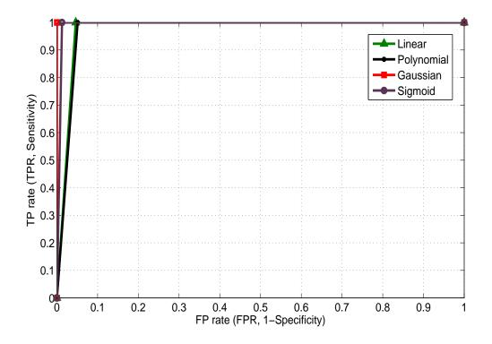
Figure 5.2: ROC curve performance of various kernel in OCSVM.
