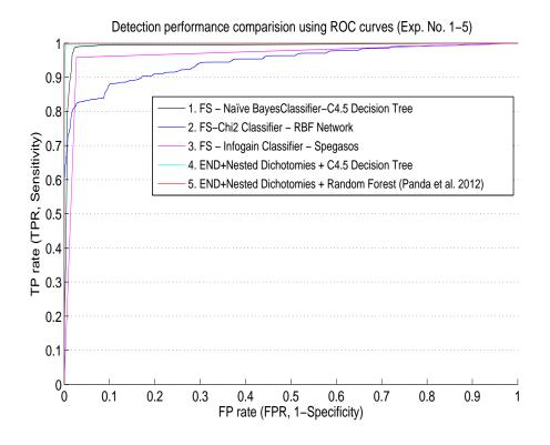
Figure 4.3: ROC curve showing Exp. No. 1-5 (2-class classification).
