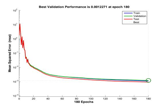
Figure 3.8: Performance of stage-2 classifier with 35 hidden layers at 180 epochs.
