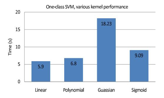
Figure 5.3: Performance of various kernel (Time complexity) in OCSVM.
