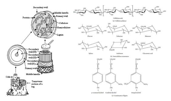
Fig. 1 Composition and chemical structure of lignocellulosic residues (Adapted from Saini et al., 2015; Sánchez, 2009)
