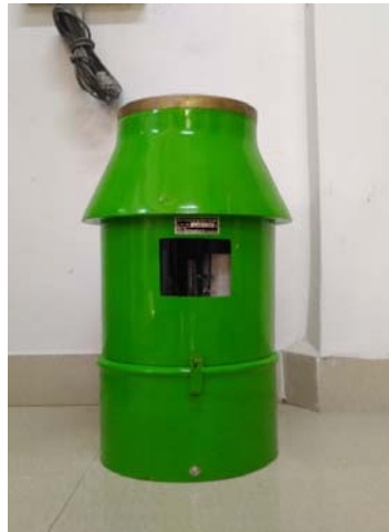
Figure No. 2: Self Recording Rain Gauge for recording rainfall data.
