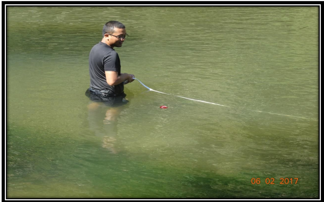
Plate 5.5.2: Tlawng river measurement by float method at Ailawng.
