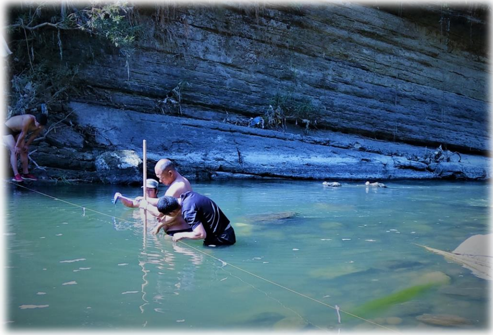
Plate G: Measuring depth across the river.
