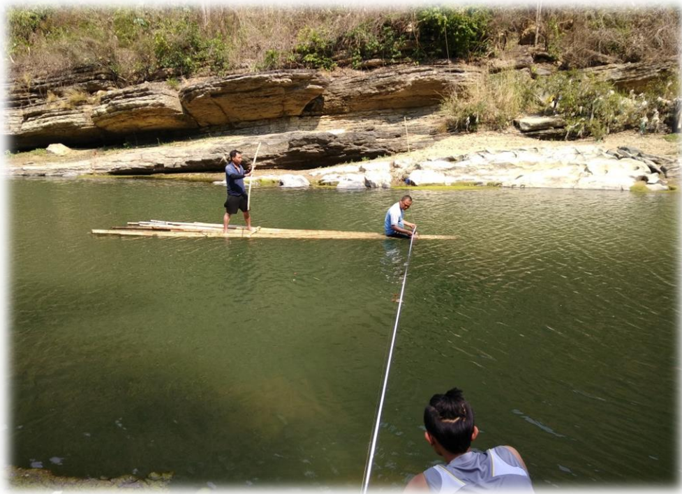
Plate E: River cross section measurement by using a bamboo raft at Ailawng.
