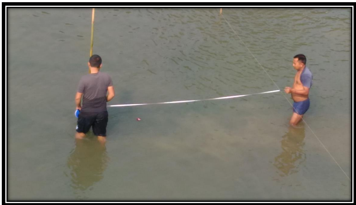
Plate 5.5.3: Tlawng river measurement by float method at Bairabi town.
