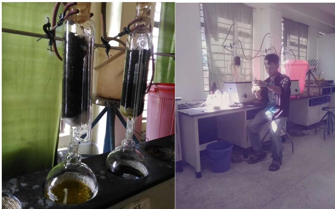
Photo 4: Extraction with soxhlet apparatus and purification of extract
