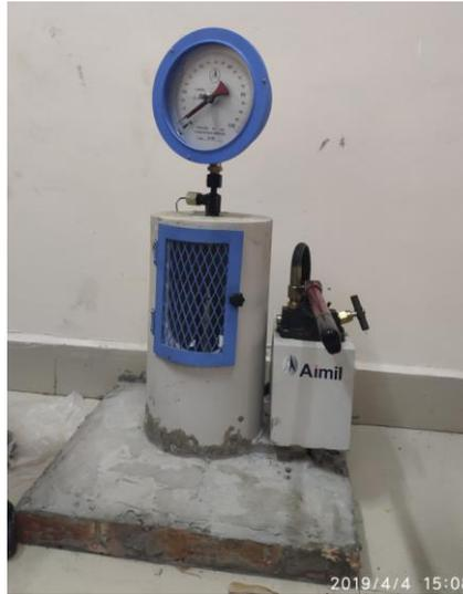
Figure 2. 3: Point load Test
