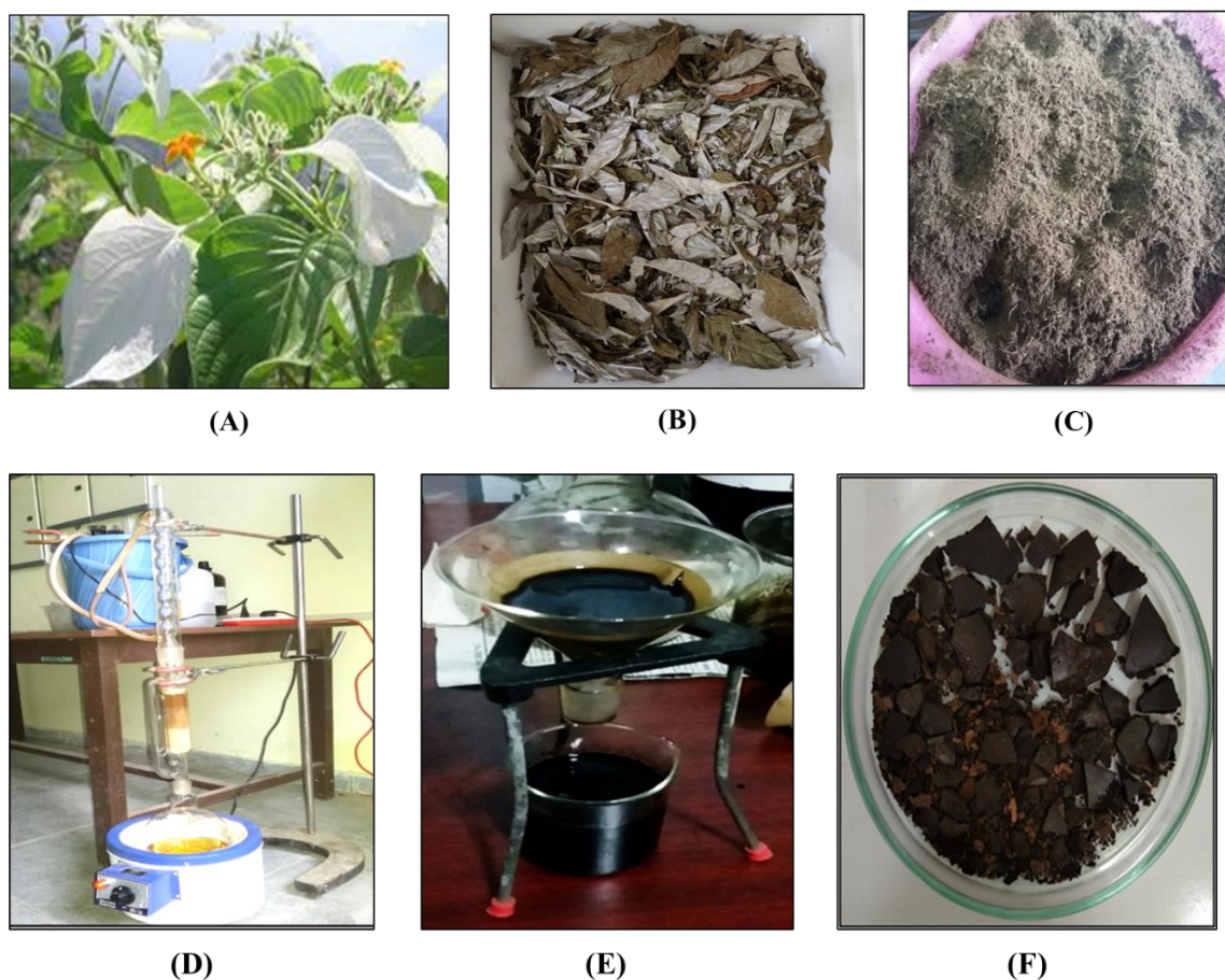
Figure 1.1. (A) Mussaenda macrophylla Wall.; (B) Dried leaves of M. macrophylla ; (C) Powdered leaves; (D) Extraction using soxhlet apparatus; (E) Filtered liquid extracts; (F) Dried extracts.
