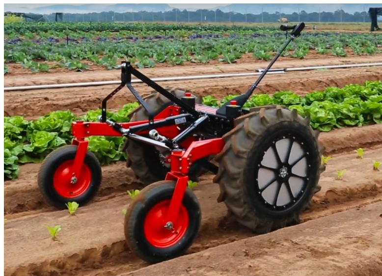
Figure 2.7 2-Wheel drive differential robot prototype (SWAGBOT)
