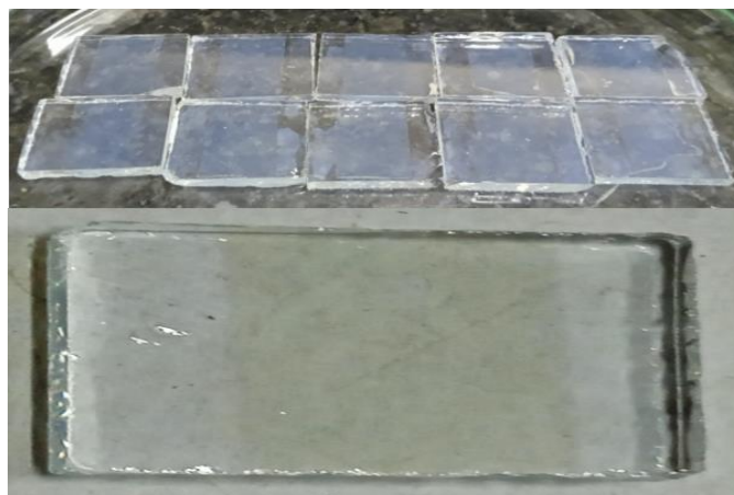
Fig. 5.9. Patterned FTO glass (ZnO dust and HCl)
