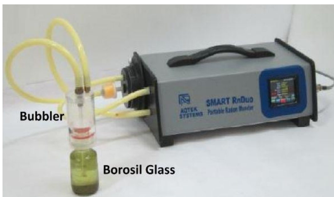
Fig. 3.6: Photo showing the arrangement of SMART RnDuo and collected water sample in a glass bottle ( 2.2 \times 10^{-4} \text{ m}^3 ) for measurement of the isotope pair data in water.
