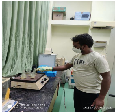
Soil sample digestion process using hot plate
