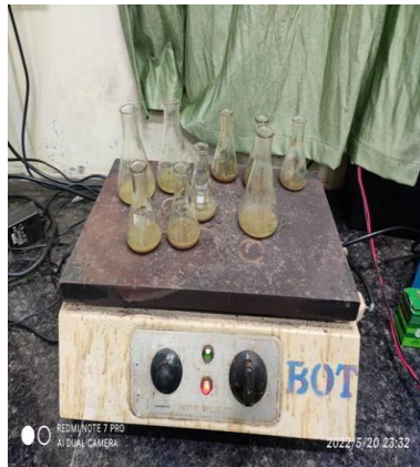
Soil sample digestion process using hot plate
