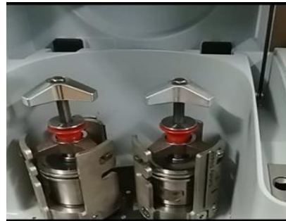
3-year annual tree ring core segment, making powder using a ball mill
