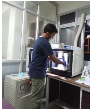
Tree ring sample digestion process using microwave digester
