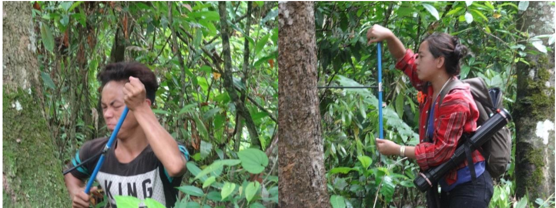
Photo plate 2: Coring of the sample trees using the Haglof Increment borer.
