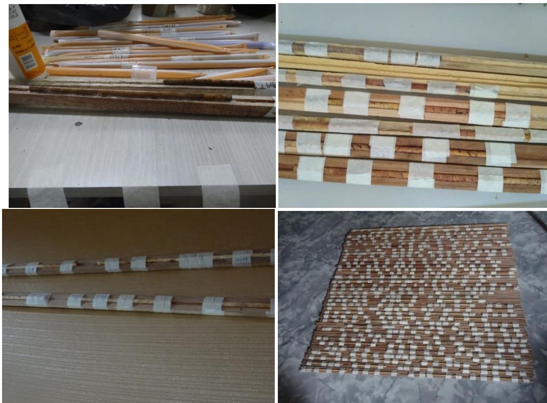
Photo plate 5: Mounting of cores on the wooden groove using the water base glue.
