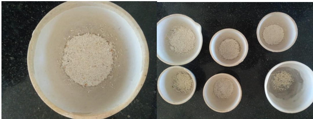
Photo plate 9: Ash of the cores for estimation of carbon concentration using dry ashing method.
