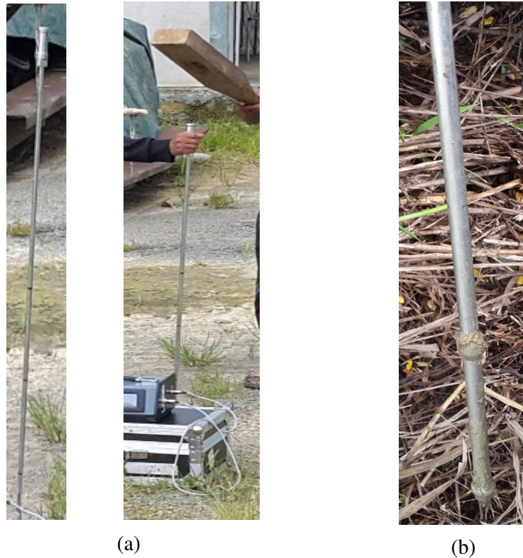
Fig. 2.17. (a) Soil probe showing the upper end and a wooden hammer. (b) Soil probe showing the lower end
