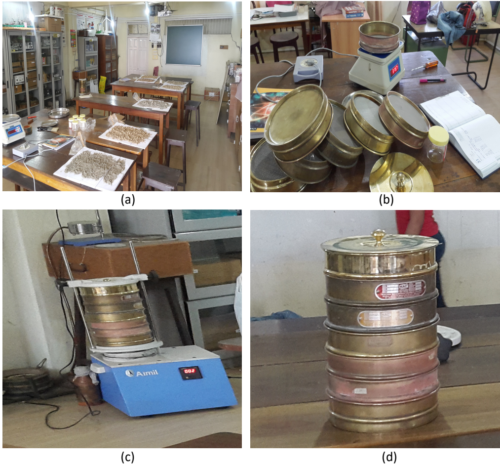
Fig. 2.6: Dressing of soil samples for Soil type and Grain size study-
