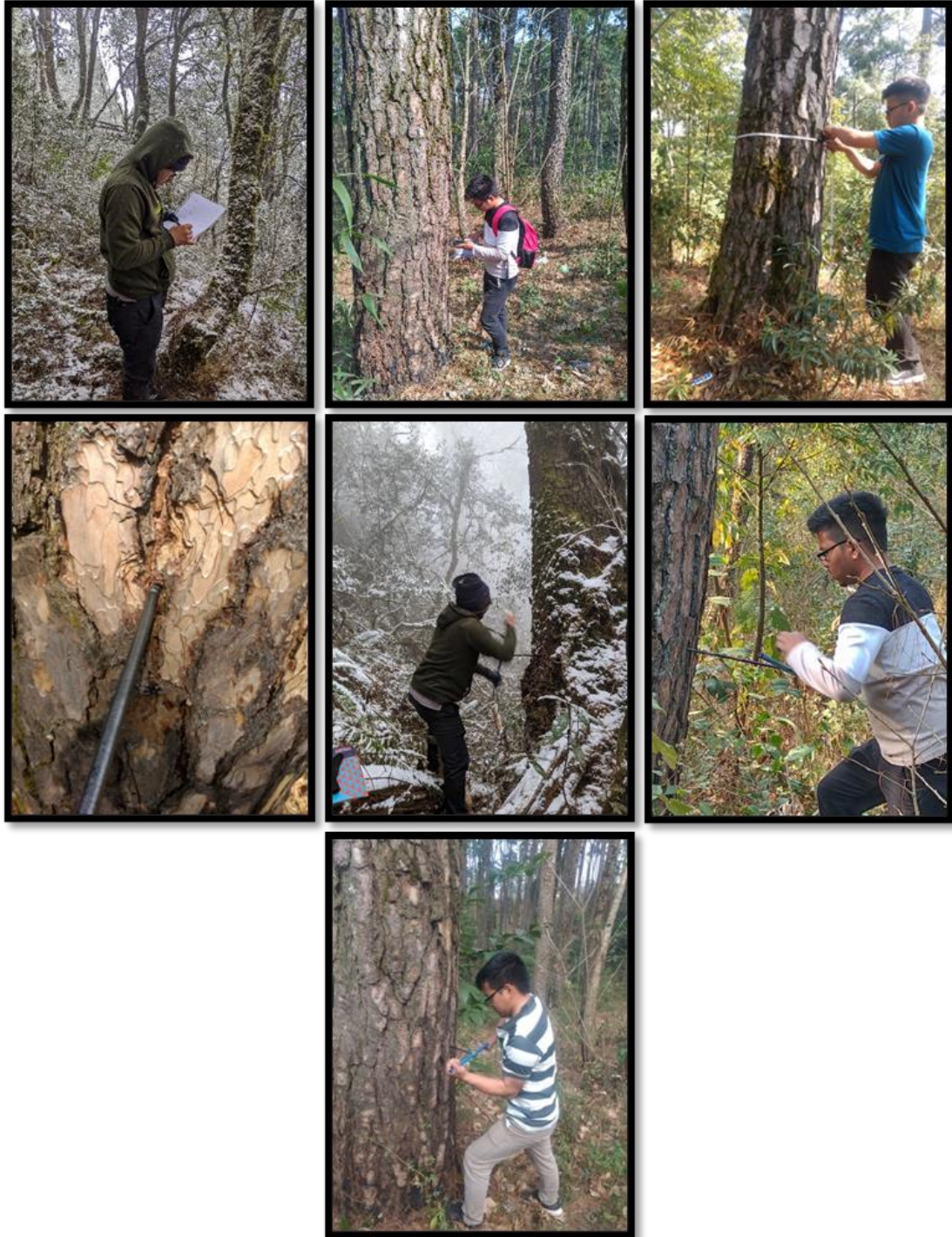
Plate No 3: Measure the DBH, taking reading of the GPS and the first step to core the tree.
