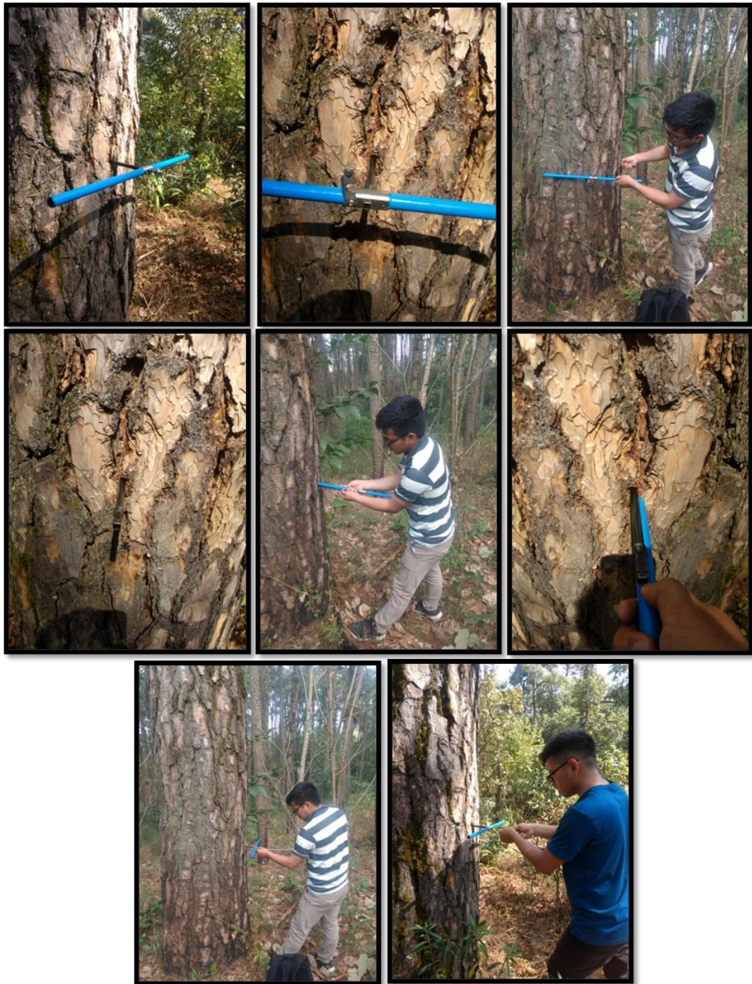
Plate No 4: Measuring how deep of the borer that are bore into the tree, if it reached to the centre the following step should be taken.
