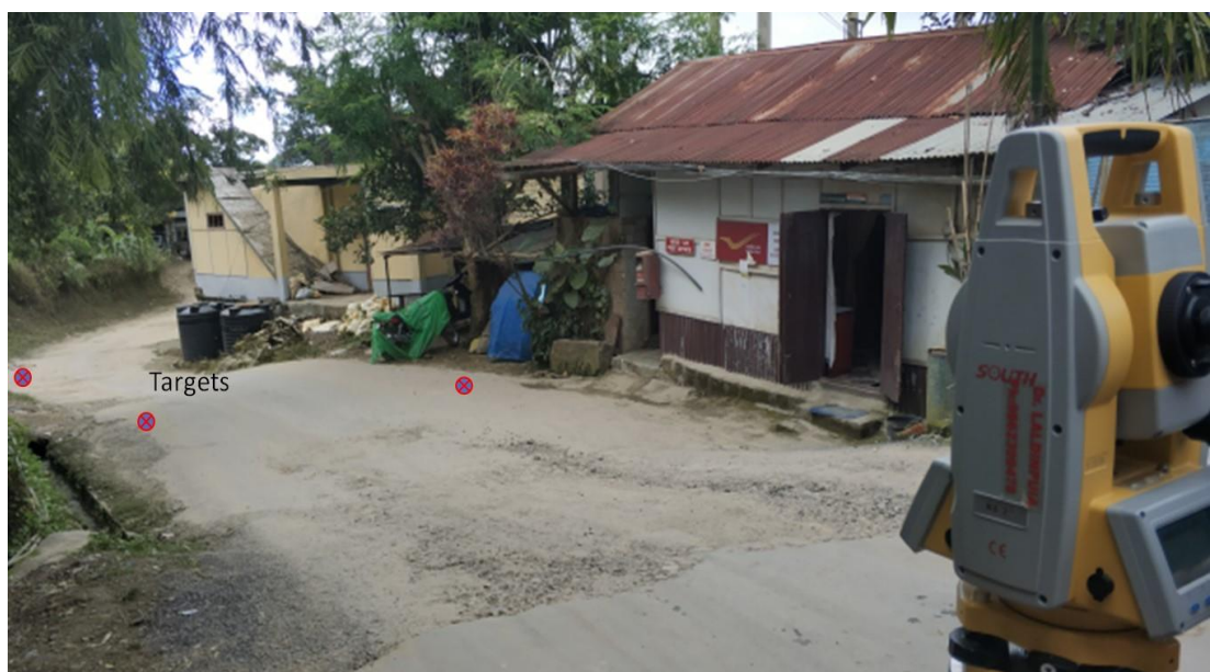
Figure 4.12: Field photograph of ground movement monitoring in location-2
