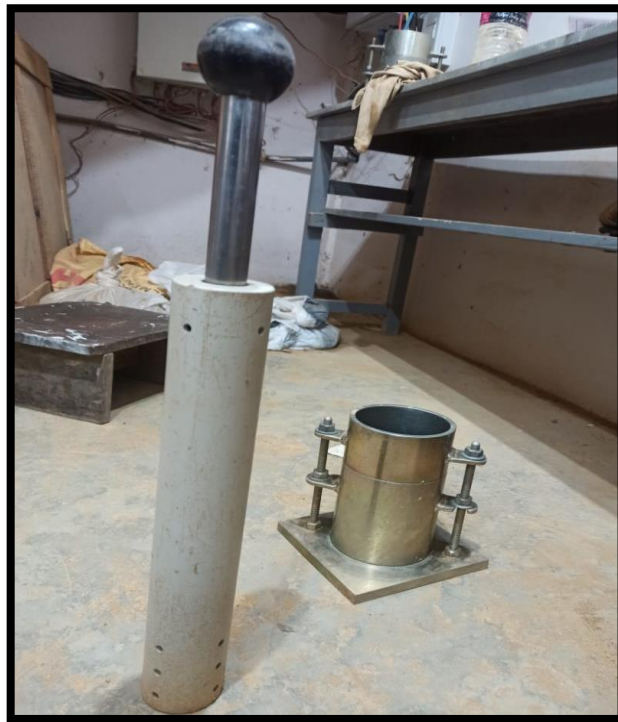
Figure 4.4: Proctor Compaction test apparatus
