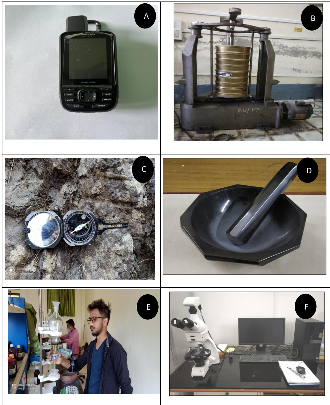
Figure 2.2. The instruments used during fieldwork and laboratory work mainly involve (A) GPS, (B) Ro-Tap mechanical sieve shaker (C) Brunton Compass (D) Agate mortar and pestle (E) Separating funnel equipment assembled for heavy mineral separation. (F) Leica-DM750P Trinocular Polarizing Microscope fitted with CCD camera.
