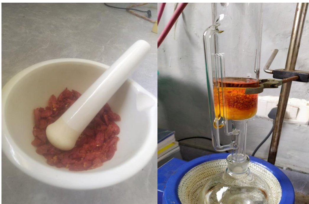
Photo plate B. Extraction of plant specimen using Soxhlet apparatus for analysis.
