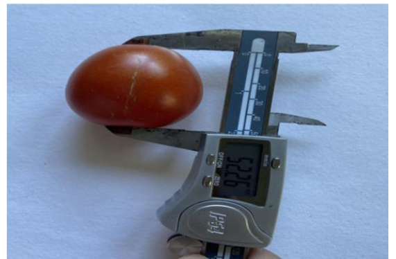
Photo plate 23. Measuring the Fruit length and fruit breadth
