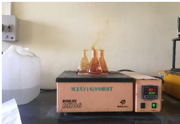
Photo plate 14. Digestion of plant samples for nutrient analysis
