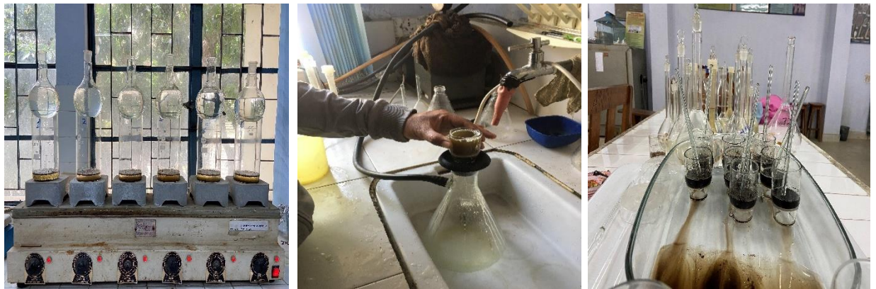
Photo plate 13. Estimation of Lignin, Cellulose and hemicellulose
