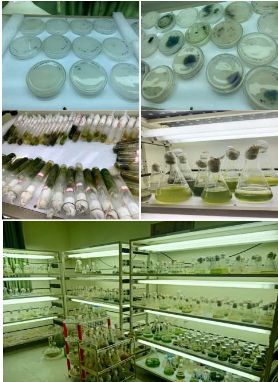
Figure 9: Laboratory cultivation of algae: from inoculation to harvesting.
