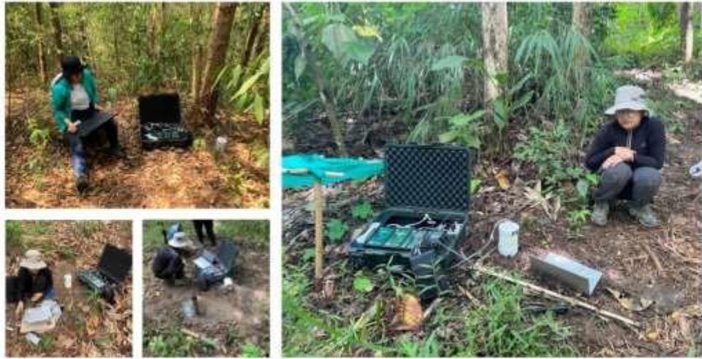
Photo plate 9: Soil respiration measured using Q-Box SR1LP.
