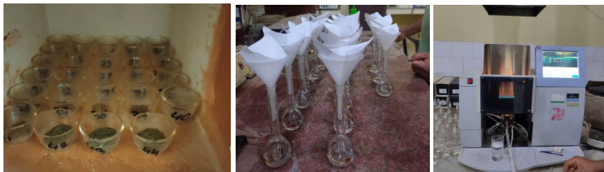
Plate 32 Estimation of mineral content by dry ashing using AAS (atomic absorption spectrophotometry)
