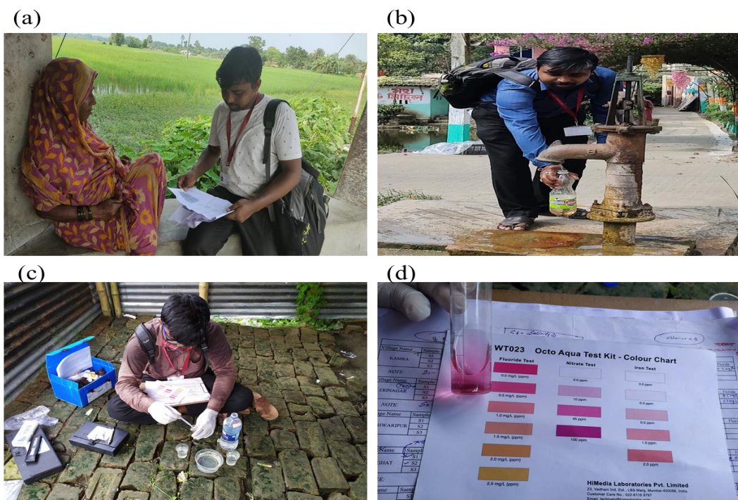
Figure 1.3: Primary survey (a) researcher is collecting household-level data, (b) the researcher is collecting samples of drinking water for testing (c) the researcher is testing water samples, and (d) the results of the water samples test; Source: By author
