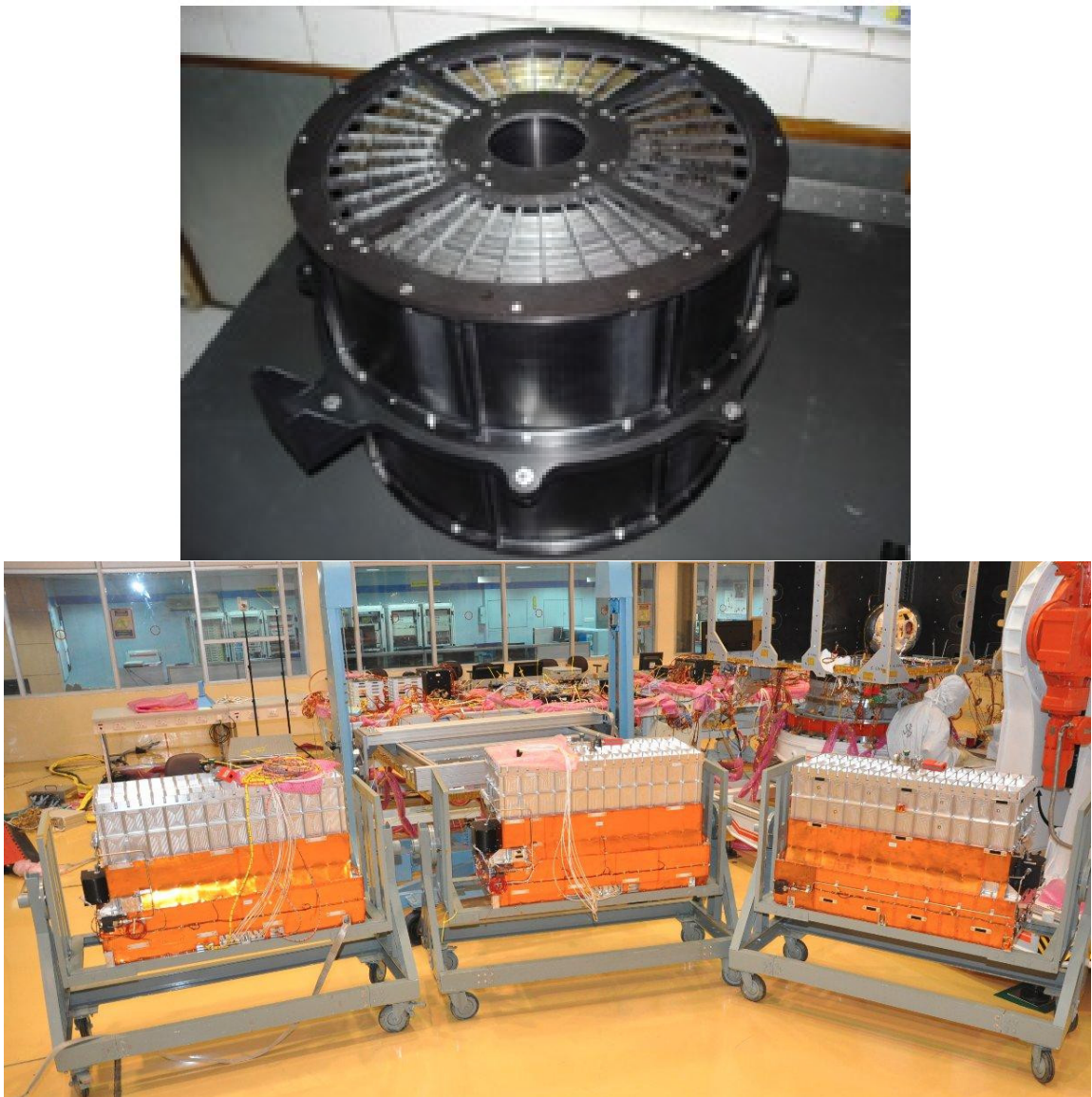
Figure 2.2: Above: Mirror assembly of SXT. Below: 3 units of LAXPC instrument at the time of integration. Pic Credit: ISRO
