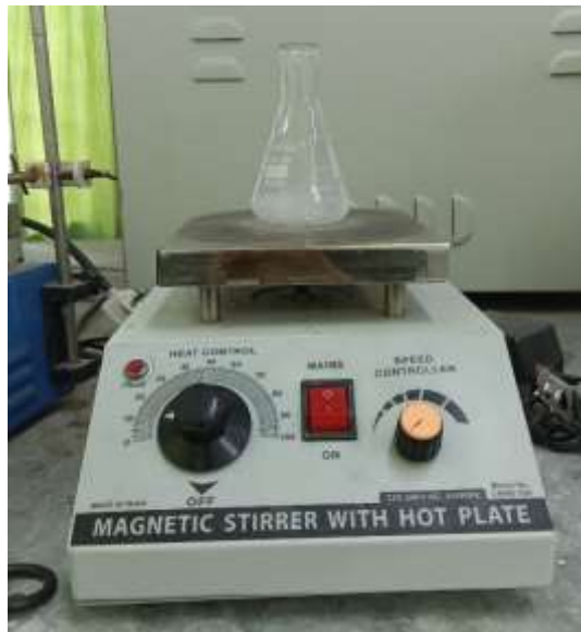
Fig. 2.1: A magnetic stirrer used to stir a mixture in the proper ratio.
