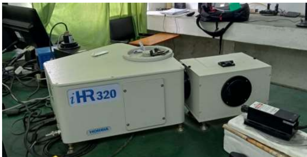
Fig. 2.10: iHR320 imaging spectrometer used for recording absorption and emission spectra.
