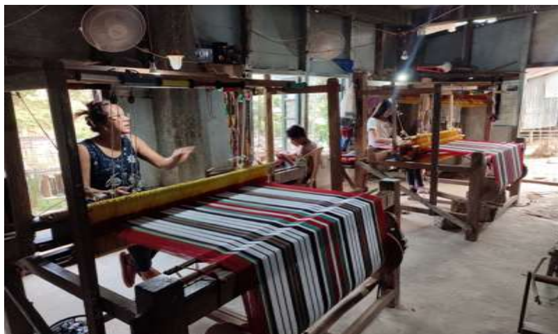
6. A respondent woman operating a mechanical handloom producing traditional Mizo fabric.
