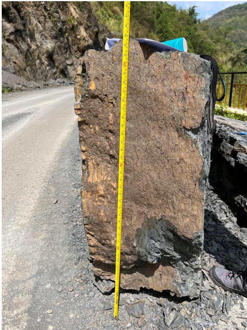
Fig. 16 Block of rock that detached from the slope bounced across the road
