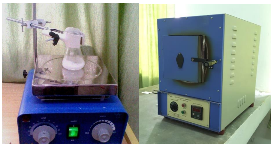
Fig. 2.1: (a) A magnetic stirrer is used to stir a mixture in the proper ratio and (b): Muffle furnace used for annealing.
