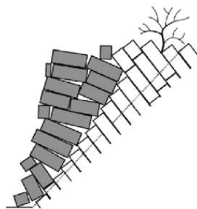
Fig: 1.4(e) Toppling failure [17]
