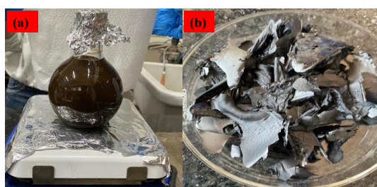
Figure 12. (a) Synthesis of GO solution (b) synthesised GO after drying
