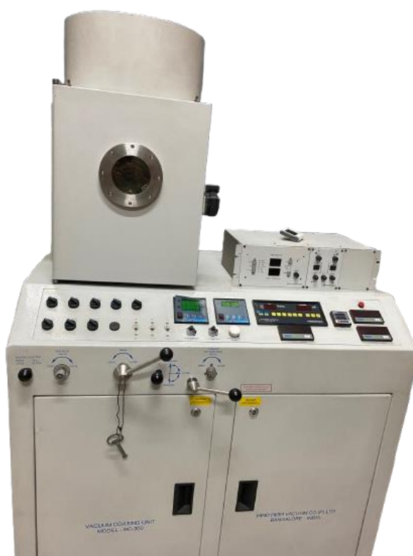
Figure 6. E-beam deposition machine used for fabrication of thin film Au electrode.
