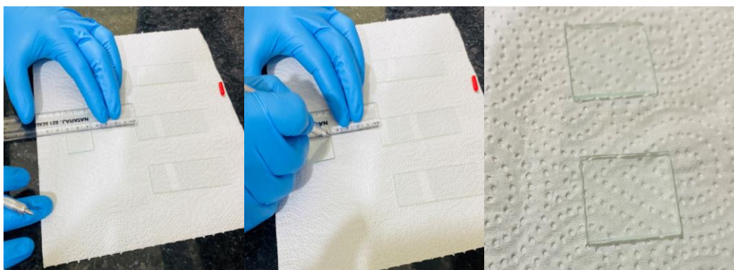
Figure 7. Microscope glass slide cutting process for fabrication Au thin film electrode.
