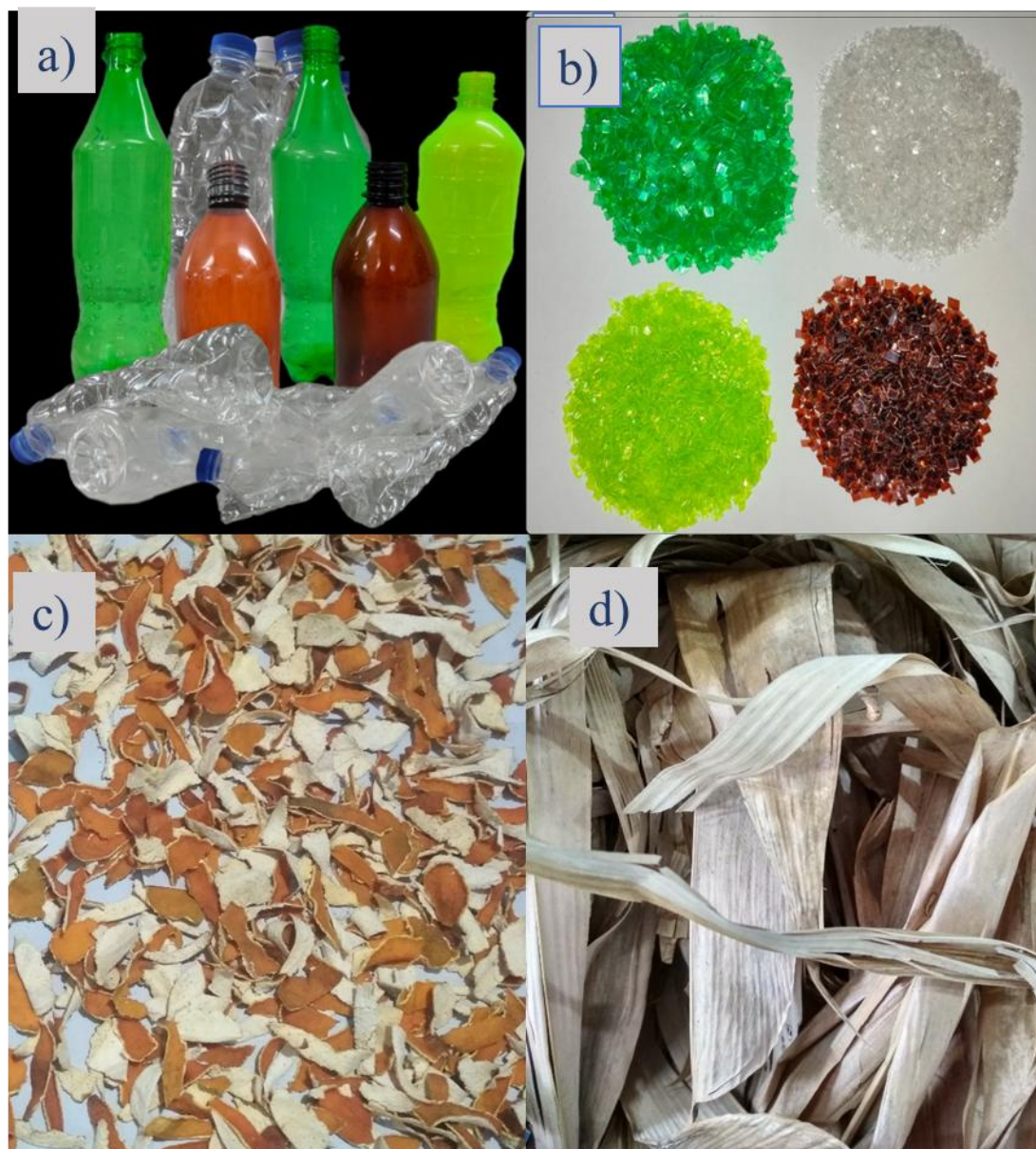
Figure 2.1: Collected samples a) color variant PET bottles, b) shredded PET flakes, c) dried orange peel, d) dried bamboo leaves.
