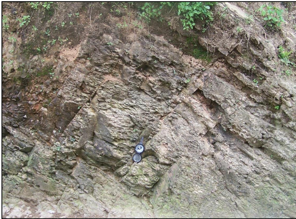
Photo Plate 3.6 A highly-jointed Shale unit
