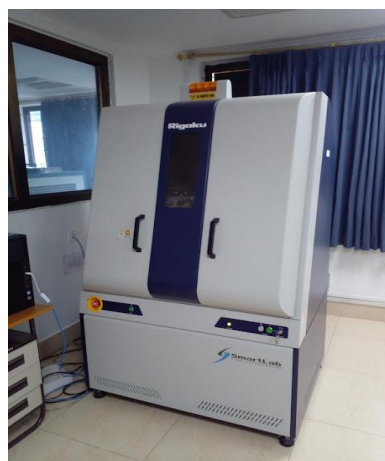
Figure 2.4: (a) Incident and diffracted radiation from crystal planes (b) Image of X-Ray diffractometer.
