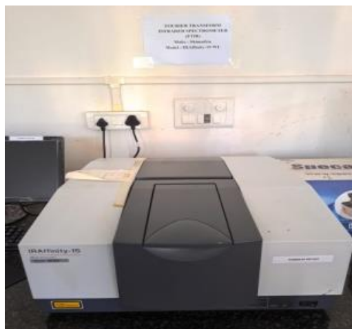
Figure 2.3: (a) Schematic diagrams and (b) Image of FTIR spectrophotometer
