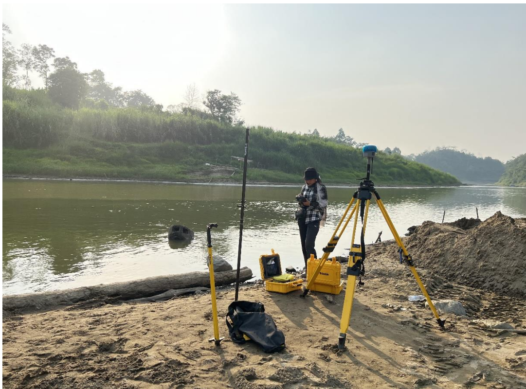
Figure 8.4 Pre- monsoon River Line Survey at Bairabi using DGPS
