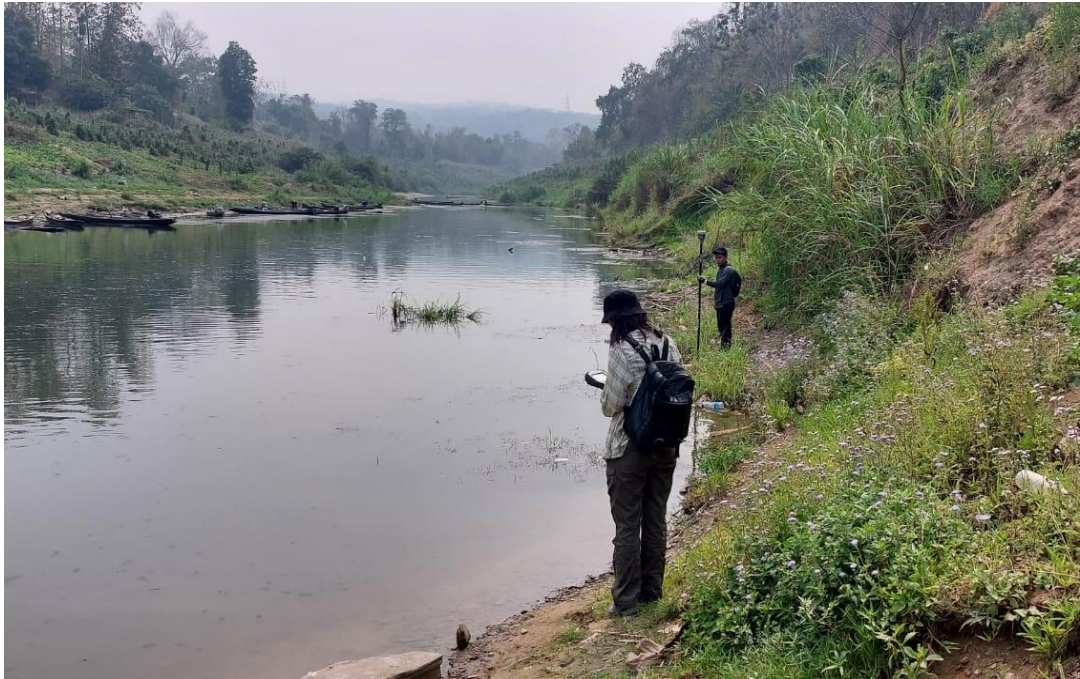
Figure 8.3 Pre- monsoon River Line Survey at Sairang using DGPS
