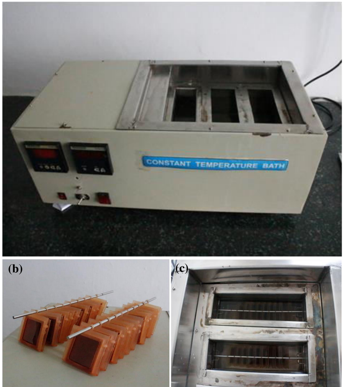
Fig. 3.8: (a) Picture of a constant temperature bath. (b) LR-115 films loaded in cartridges before etching. (c) Loaded films in NaOH solution inside the etching vessels.
