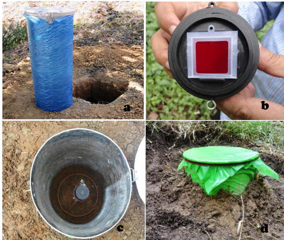
Fig. 3.5: Methods of measurement in soil. (a) Bore hole at a depth of 80 cm below soil surface. (b) LR-115 loaded in the dosimeter. (c) Loaded dosimeter inserted in a metallic cylinder. (d) The metallic cylinder sealed by a plastic cover.
