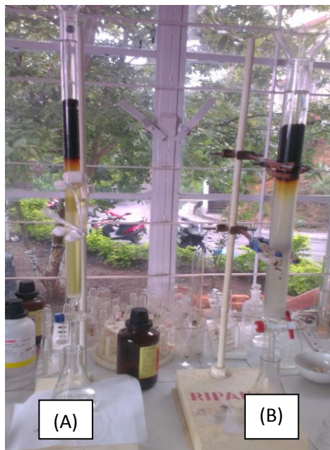
Figure 2.3. Photograph of column chromatography using silica gel as stationary phase (A) mesh 100-200 and (B) mesh 60-120
