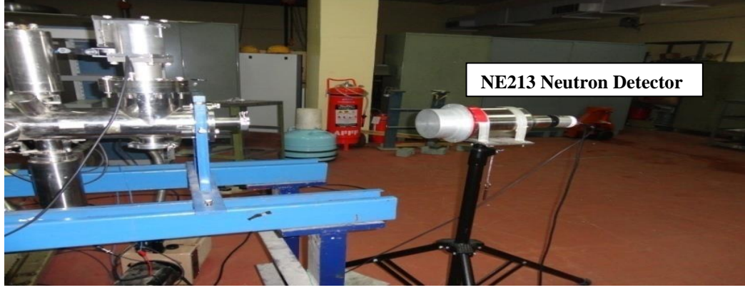
Figure 10: Experimental Setup-1: NE213 neutron detector at zero degree kept at 1 m distance from the lithium target.
