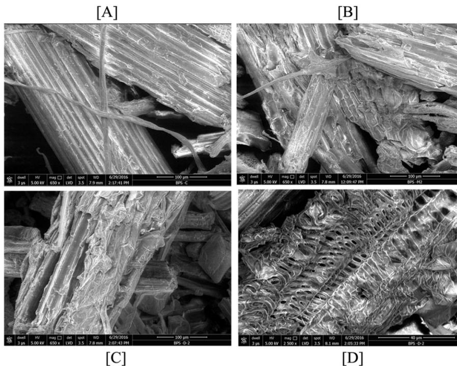
**Fig 9.** Surface destruction images of *T. latifolia* (BPS-G104) using SEM. (A) pre-treated biomass as control (BPS-C); (B) biomass treated with *Aneurinibacillus aneurinilyticus* strain DBT87 (BPS-M2); (C) and (D) biomass treated with *Serratia rubidaea* strain DBT4 (BPS-D2).
