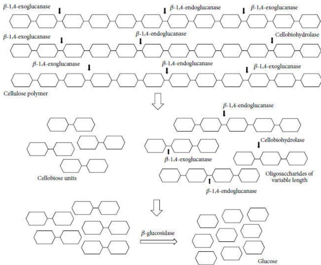
**Fig. 2** Scheme of cellulose hydrolysis (Adapted from Saini et al., 2015).
