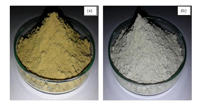
Fig 2.1. (a) Bentonite Clay, and (b) Local Clay.
