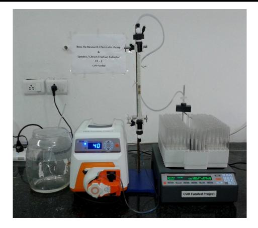
Figure 2.2. Experimental setup of column reactor.
