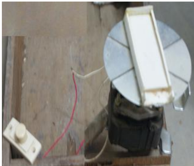
Figure 2.25: Experimental setup of spin coater.
