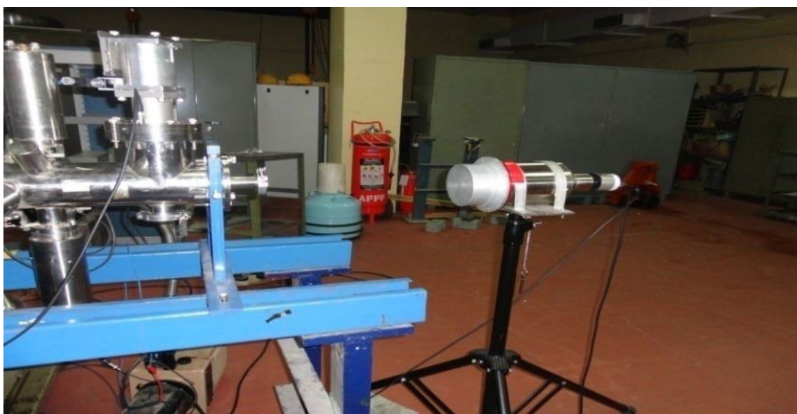
Figure 17: NE213 neutron detector at zero degree kept at 1 m distance from the lithium target.
