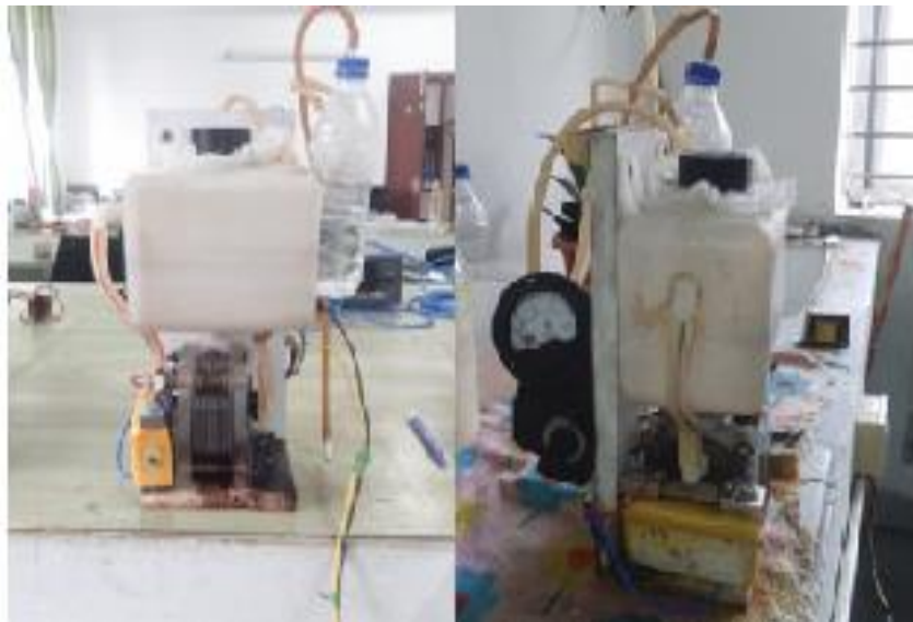
Figure 2.10: Experimental set-up for production of HHO gas
