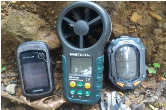
a. GPS (Garmin etrex 30), Anemometer and Barometer
