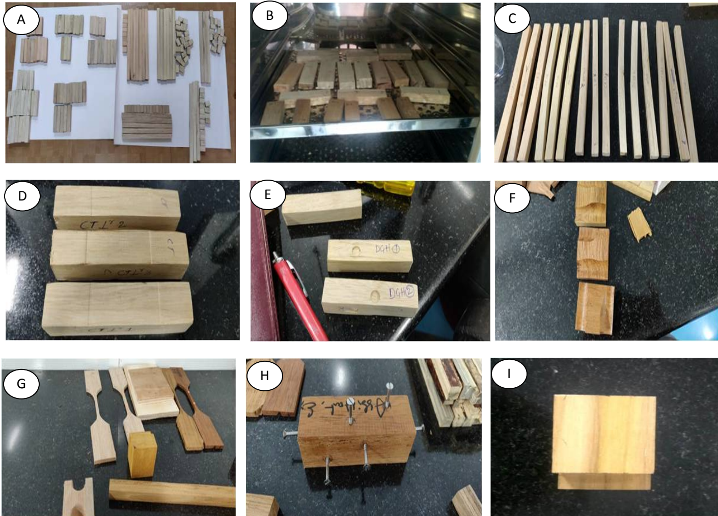
Figure 3.3. Samples for various physical and mechanical tests; A- Compression parallel, B- Moisture content and density, C- Static bending, D- Compression, E- Hardness indentation F & G- Tension, H - Screw holding power, I - Shear
