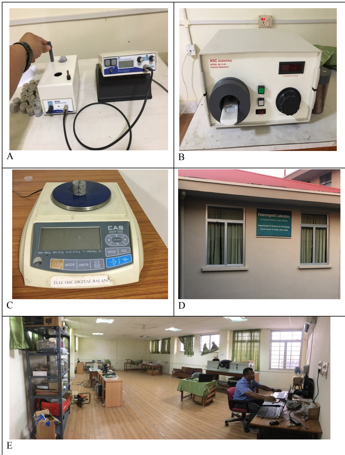
Fig.3.6. (c) Laboratory photographs: A) Bartington MS2 Magnetic susceptibility meter. B) ASC Scientific Impulse magnetizer. C) Electronic Digital balance. D) Paleomagnetic laboratory, Dept of Geology, MZU E) Panoramic view of laboratory.
