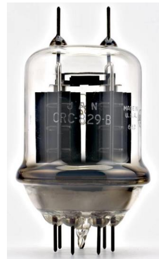
Figure 3.3: (a) Schematic diagram of pentode, (b) Photograph image of 829B power tube.
